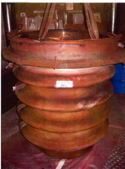
Fig. 9. A bellows tested on Superphenix heat exchanger.
