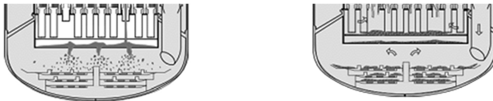
Figure 9 : JSFR multilayered core catchers – Left: sketch of relocation phase – Right: Sketch of DHR phase (Matsuba et al., 2012)
